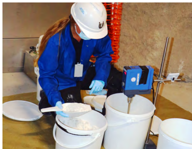
In the Mont Terri Rock Laboratory, mortar is mixed for the experiment.
