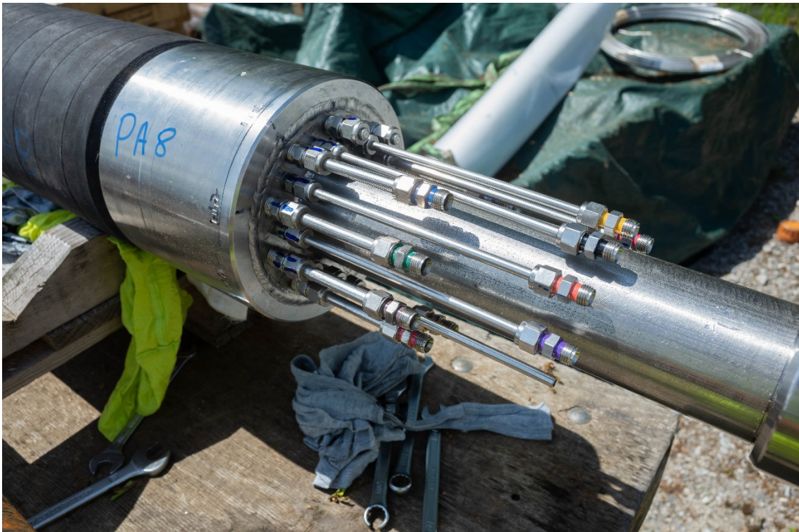
Fig. 2-3: Connections of monitoring and packer inflate lines on packer 8 Lines are identified by a colour code
