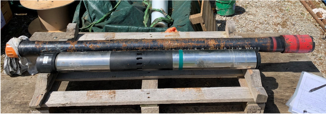
Fig. 2-5: Sliding sleeve with a 1 m section of a pup joint behind
