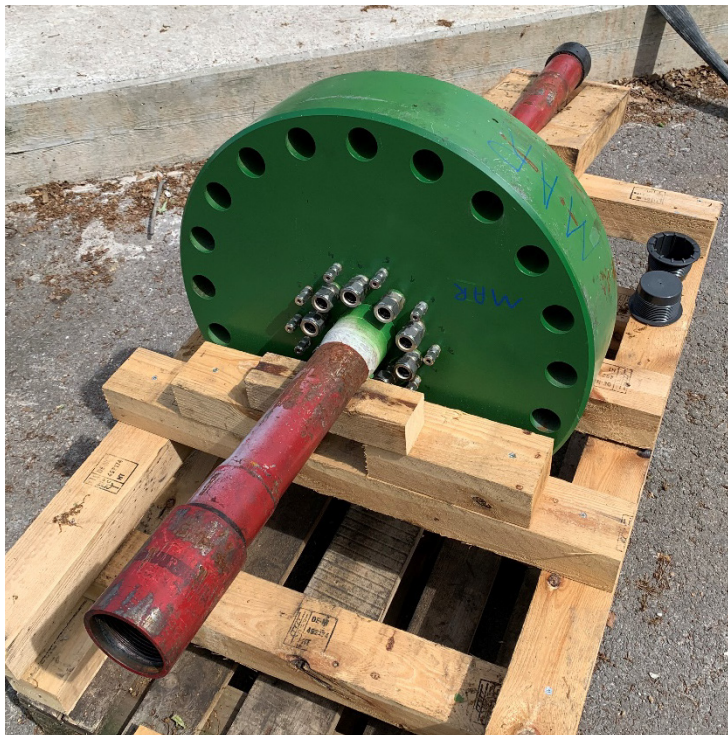
Fig. 2-8: Landing spool with fittings for standpipes and packer inflate lines
