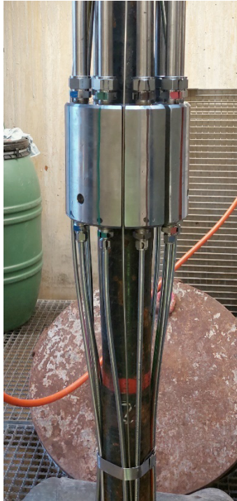
Fig. 2-1: Central tubing with monitoring and inflation lines below the hanger sub and standpipes above the hanger sub
