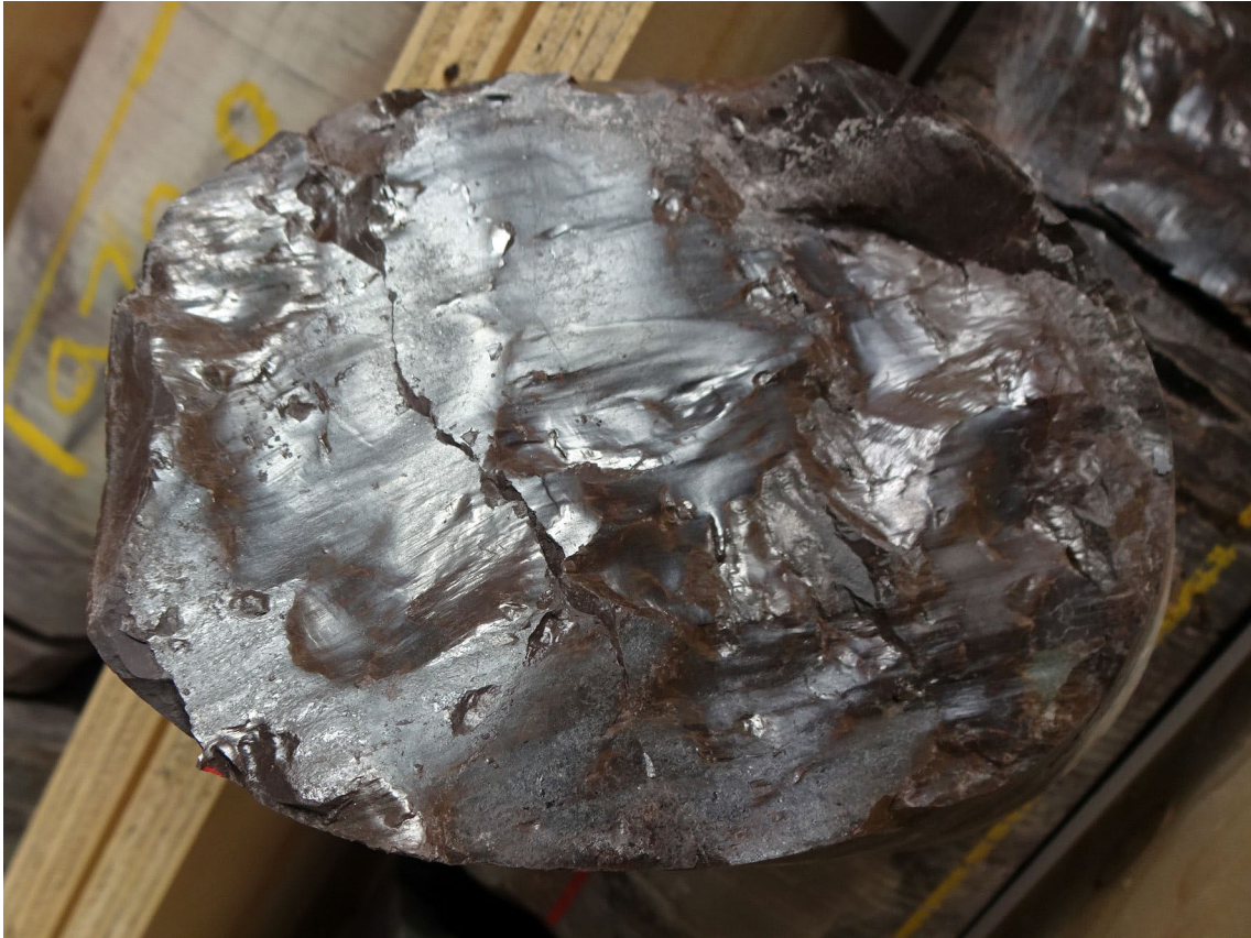
Fig. 3-5: Mirror-like fault plane
