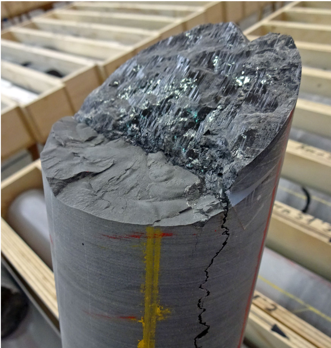
Fig. 3-6: Stylolitic fault plane
