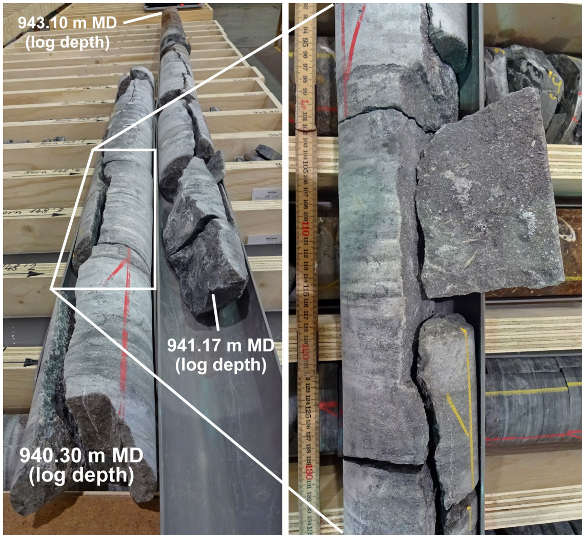
Fig. 5-4: Partly open fractures within the Staffegg Formation from 940.30 m to 943.10 m MD (log depth)
