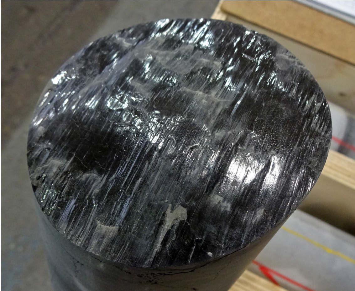
Fig. 3-4: Mirror-like fault plane
