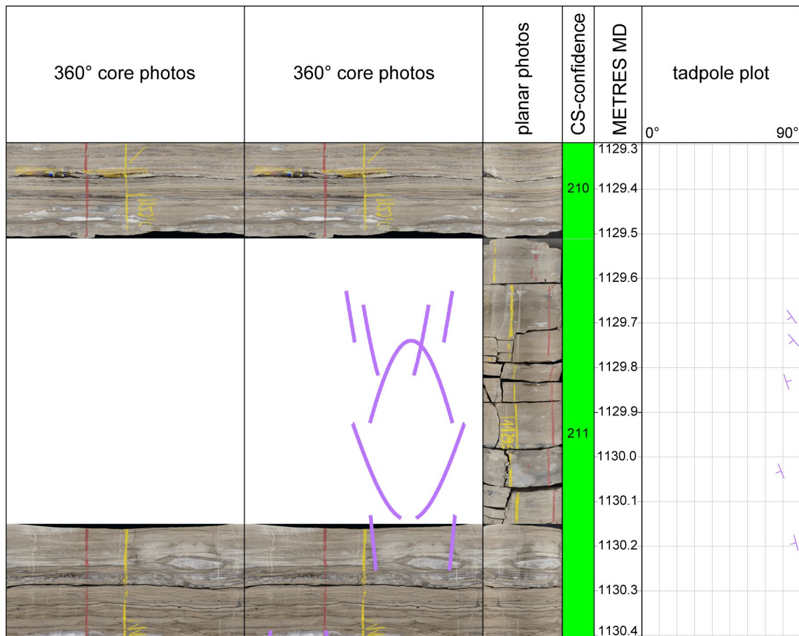
Fig. 2-5: Interval without 360° core photographs from 1'129.50 m to 1'130.15 m MD (log depth) in the Zeglingen Formation
