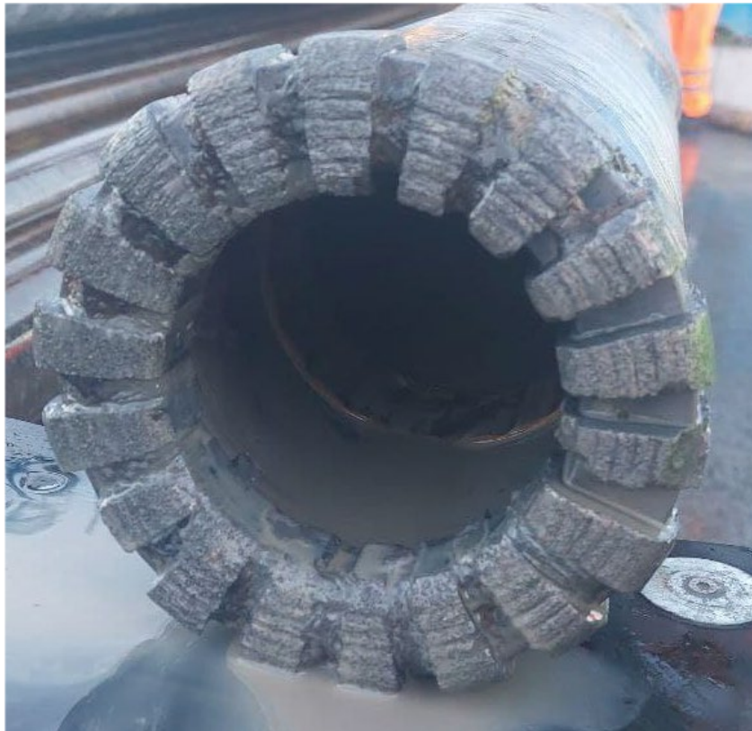
Fig. 3-13: Impregnated core bit after POOH from a depth of 979 m MD
