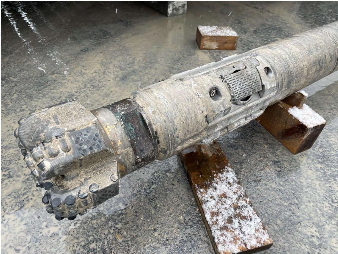
Fig. 3-8: RSS system and PDC bit after POOH from a depth of 577 m MD
