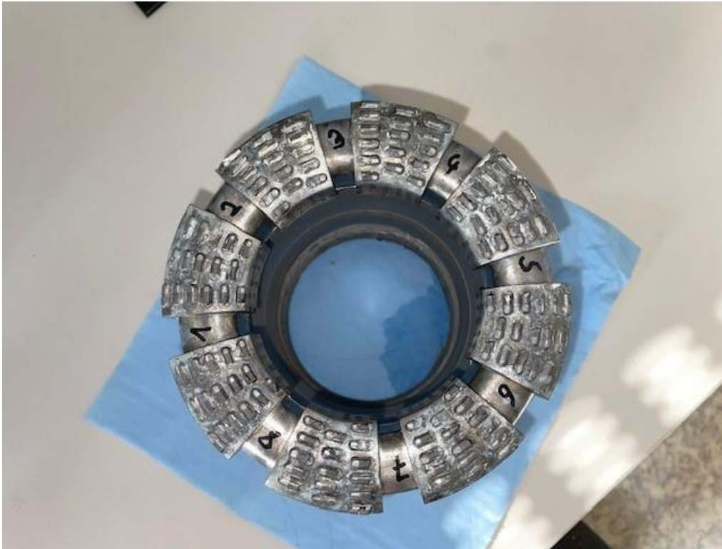
Fig. 3-5: Synset core bit after POOH from a depth of 832 m MD
