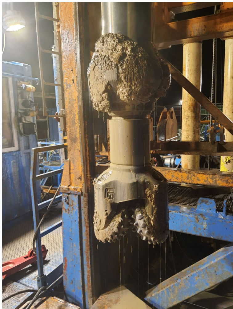
Fig. 3-3: 17½" tricone bit and 9⅝" mud motor after POOH at 350 m MD
