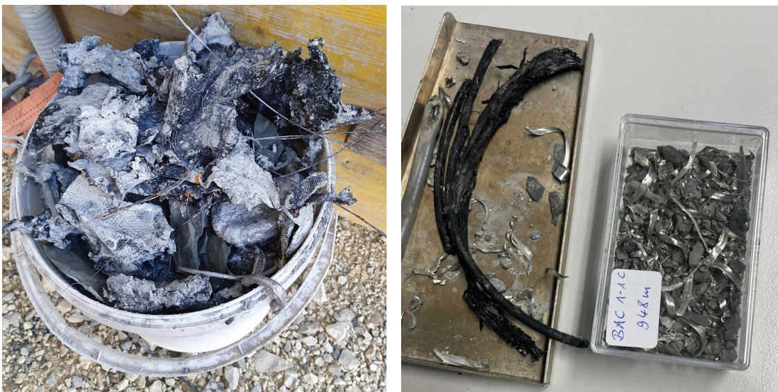
Fig. 3-12: Rubber, aluminium and steel parts from the milled dilatometer tool
