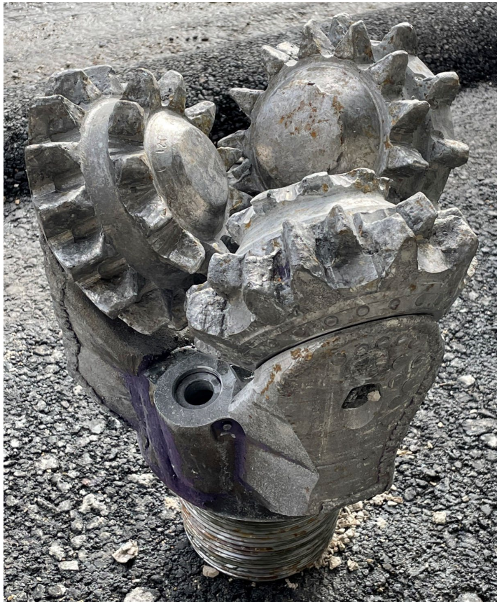
Fig. 3-10: 12¼" mill tooth bit after POOH from 947.5 m MD
