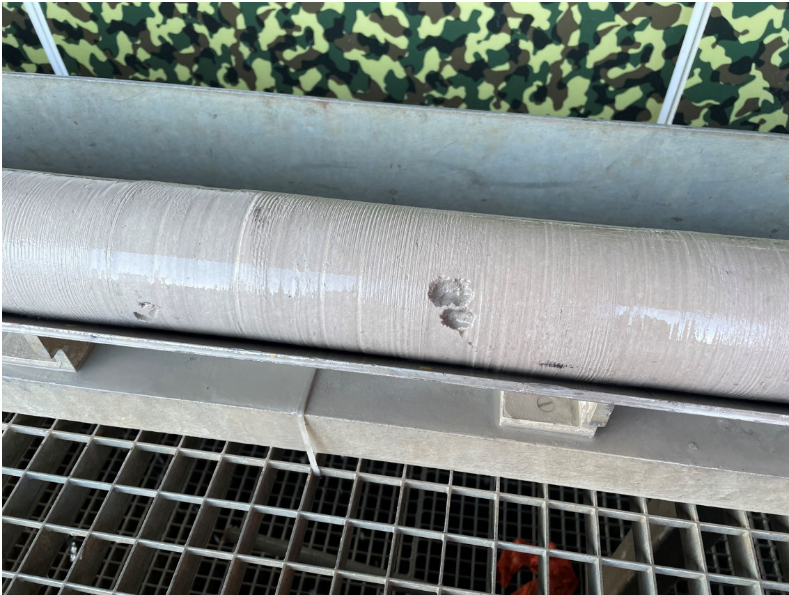
Fig. 3-9: 100% cement core from 651 m till 654 m MD
