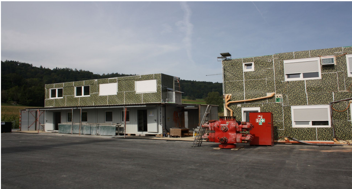
Fig. 3-19: Camouflage panels on the containers at the north-western side of the drill site
