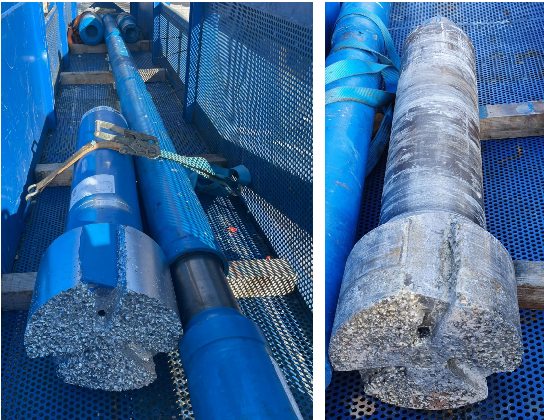
Fig. 3-11: 12 1/4" junk mill assembly before (left) and after (right) milling the dilatometer tool
