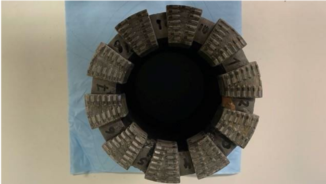
Fig. 3-7: Synset core bit after POOH from a depth of 952 m MD
