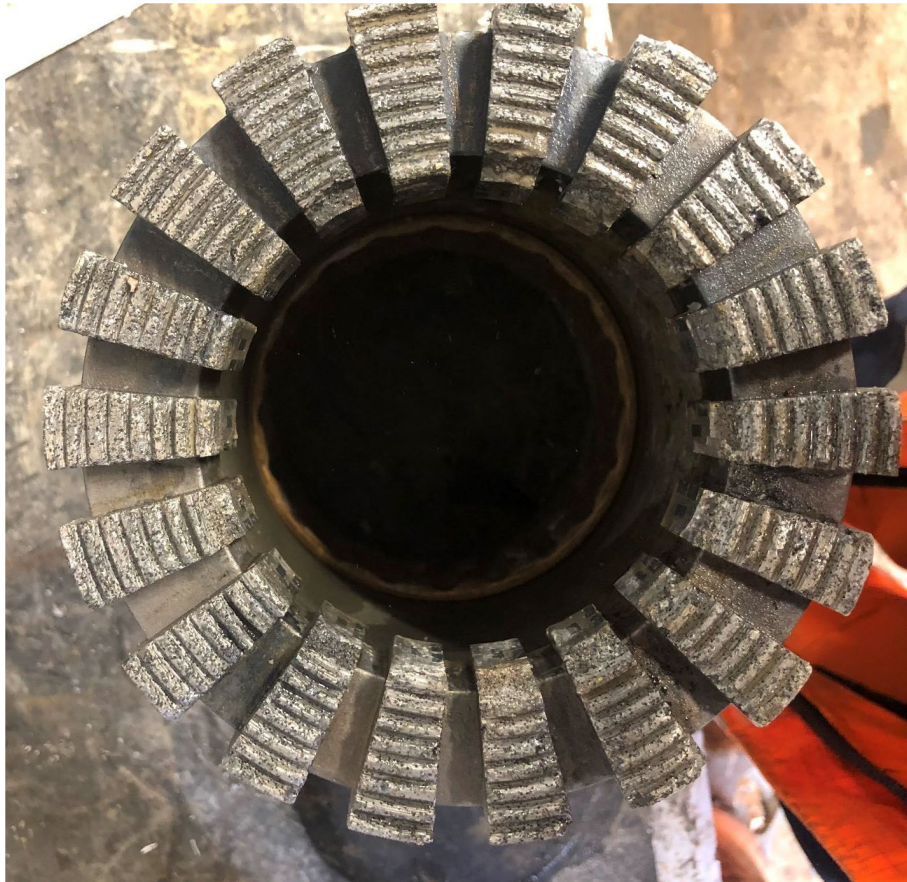
Fig. 3-14: Impregnated core bit after POOH from a depth of 1'057 m MD
