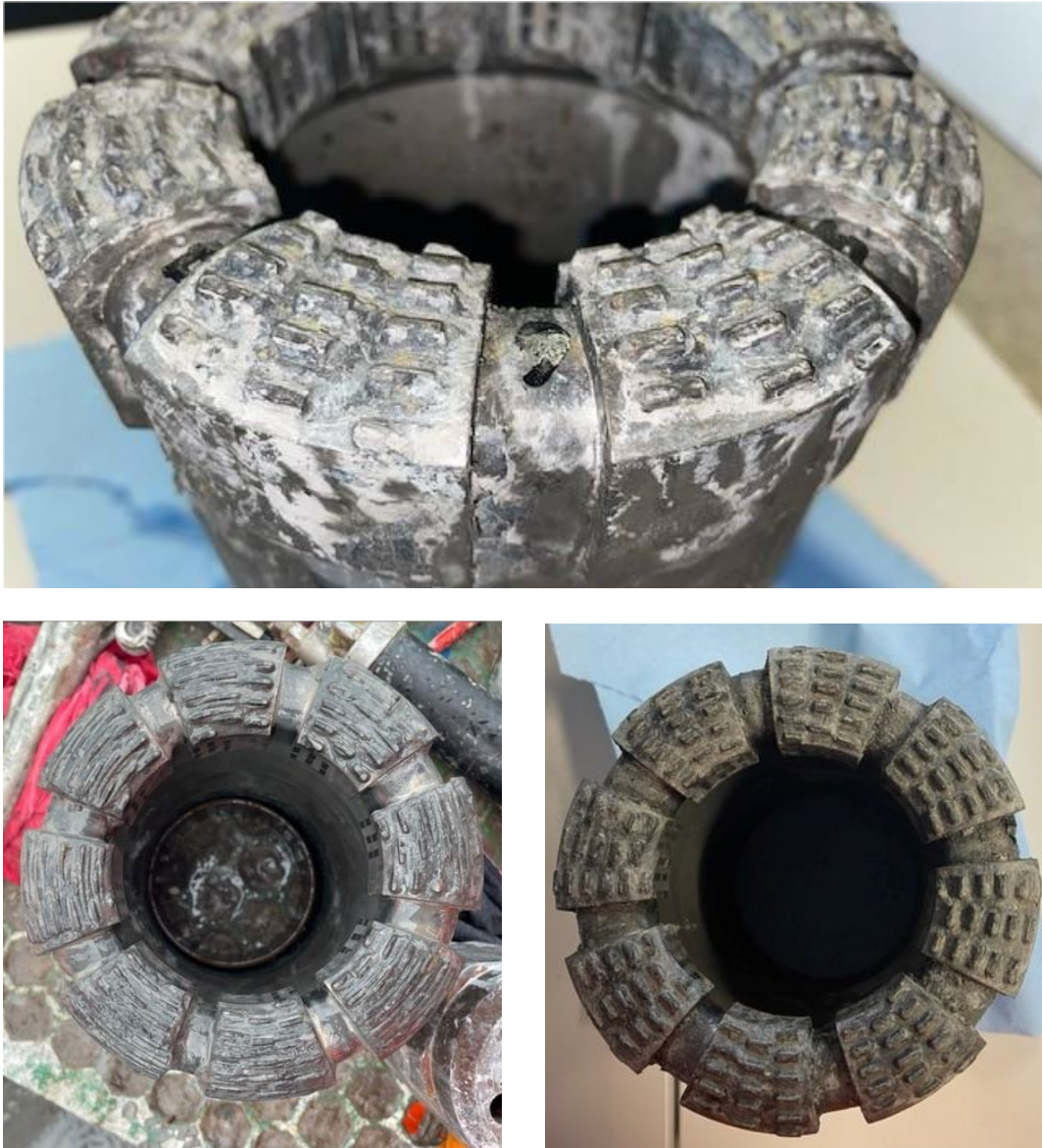
Fig. 3-6: Synset core bit after POOH from a depth of 901 m MD
