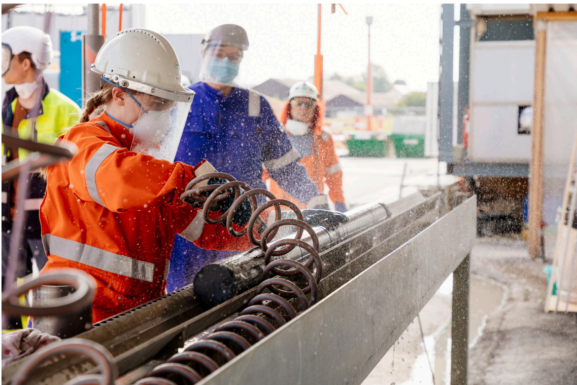
Fig. 2-4: A core is washed with water on the core processing table to remove the drilling fluid
