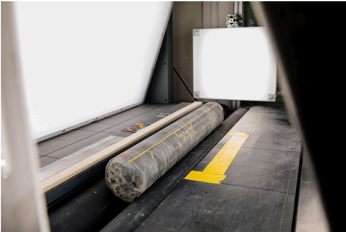
Fig. 2-9: CoreScan 3 system setup during core photography with a metre scale, a BST14 grey-scale chart and an X-Rite ColorChecker Classic Mini colour chart
