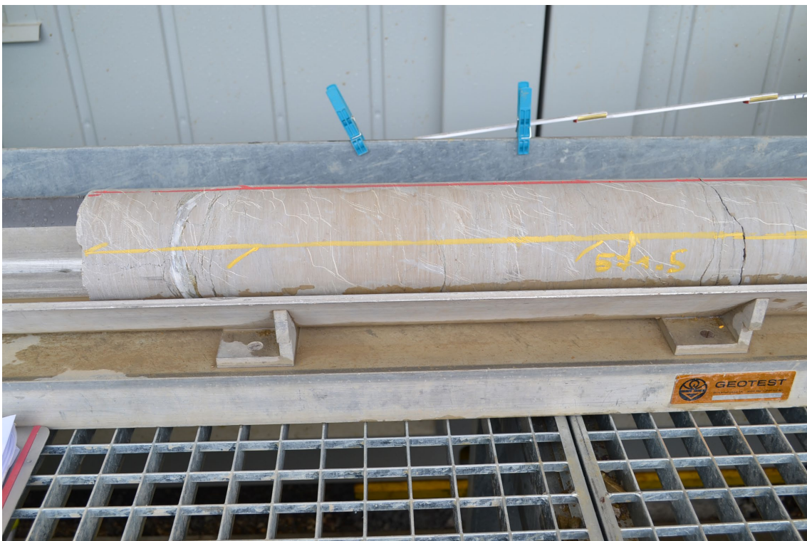
Fig. 2-6: Cleaned, measured and marked core
