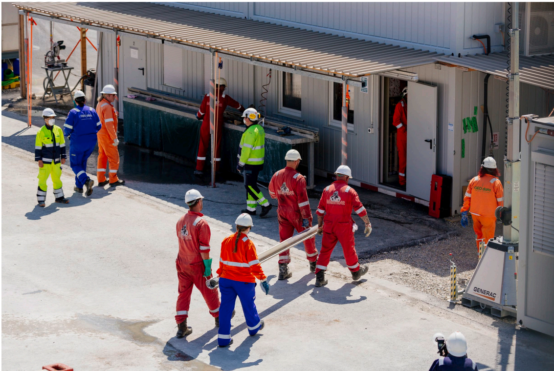
Fig. 2-2: The 3 m core in the plastic liner is carried to the core processing area
