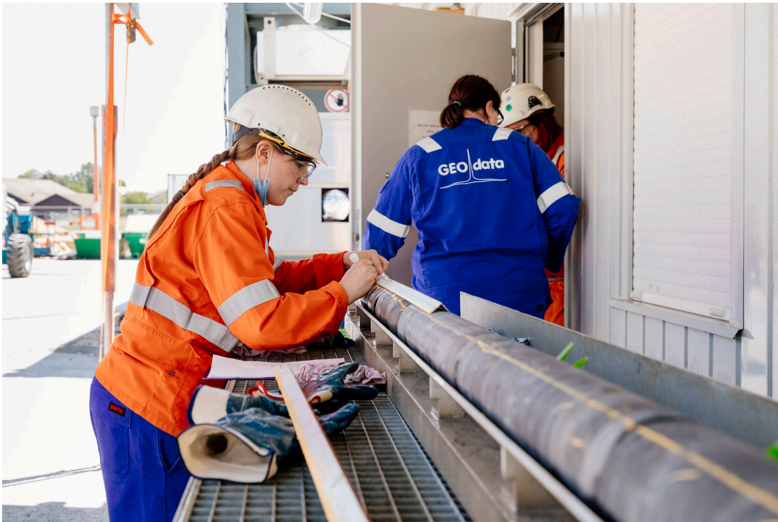
Fig. 2-5: A core is marked with orientation lines
