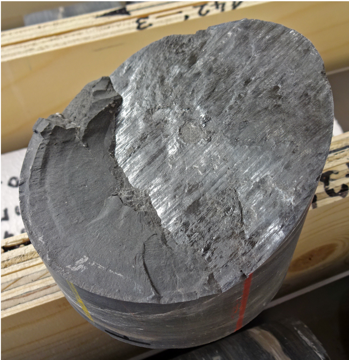
Fig. 5-5: Example of a fault plane, depth 855.61 m MD (log depth)
