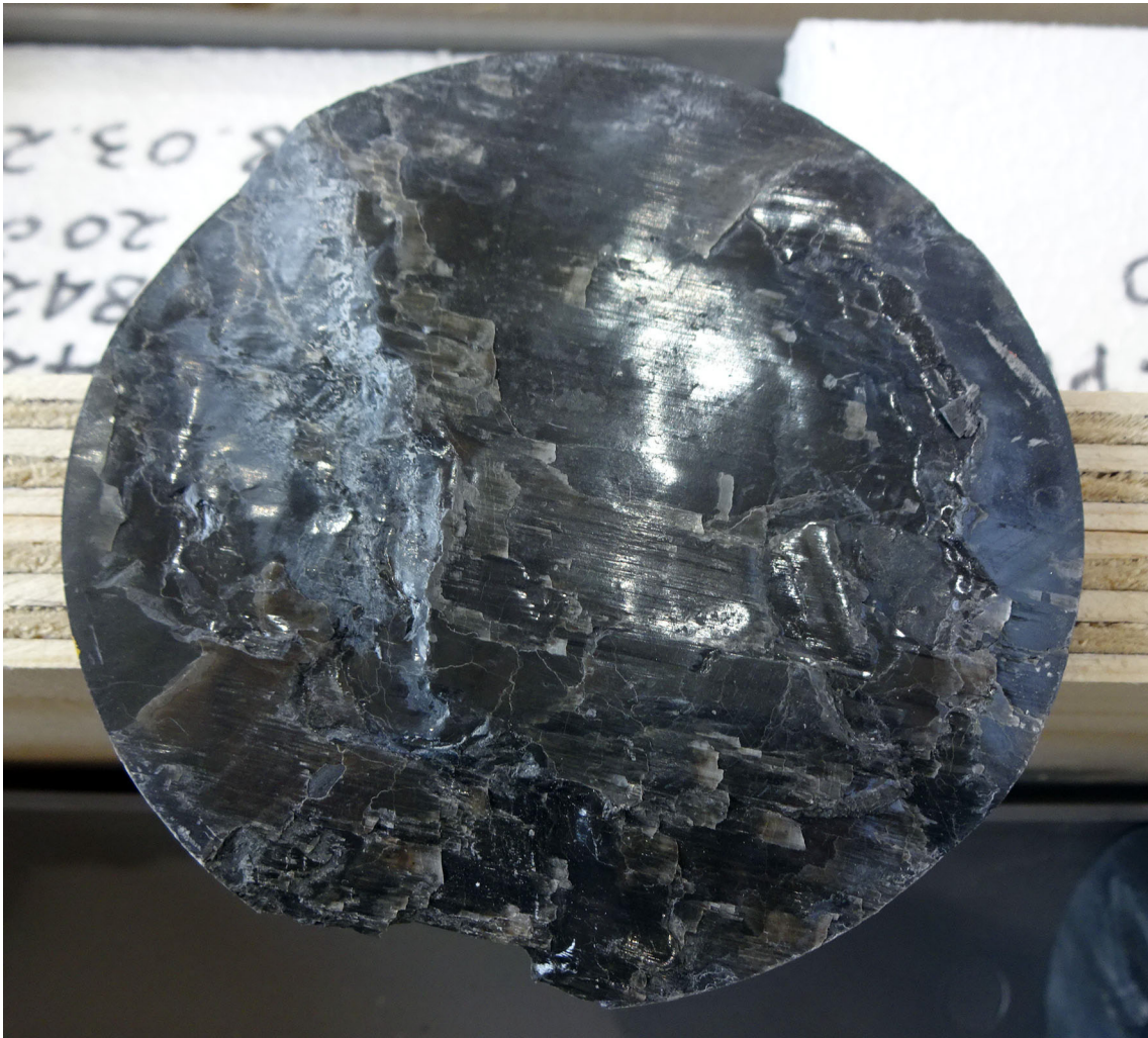
Fig. 3-5: Mirror-like fault plane
