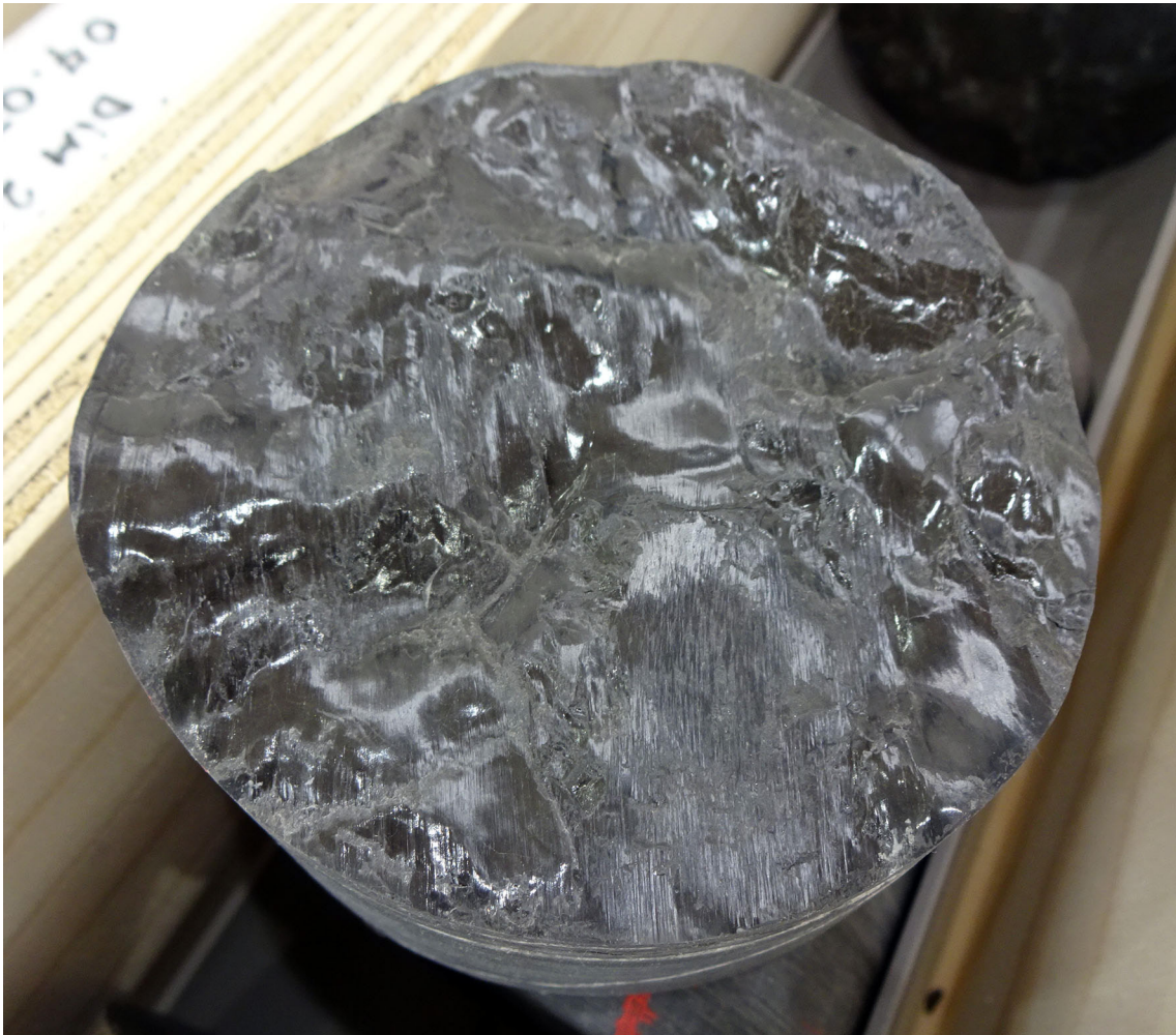
Fig. 3-4: Mirror-like fault plane
