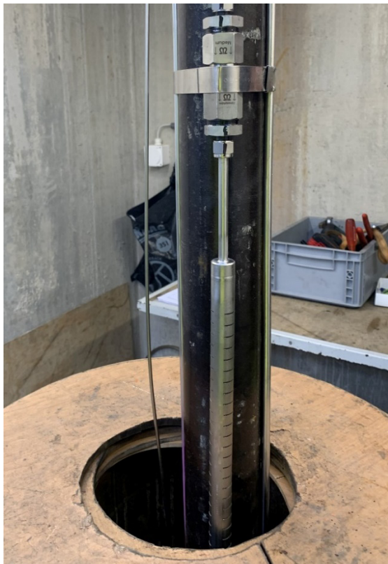
Fig. 2-5: Filter port with burst disc above, installed on the central tubing with metal banding straps
