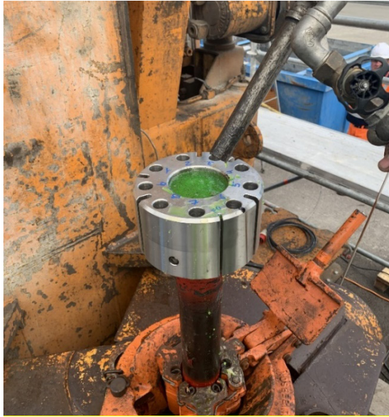
Fig. 2-1: Hanger sub with threads for monitoring and inflation lines below and standpipes above, respectively
