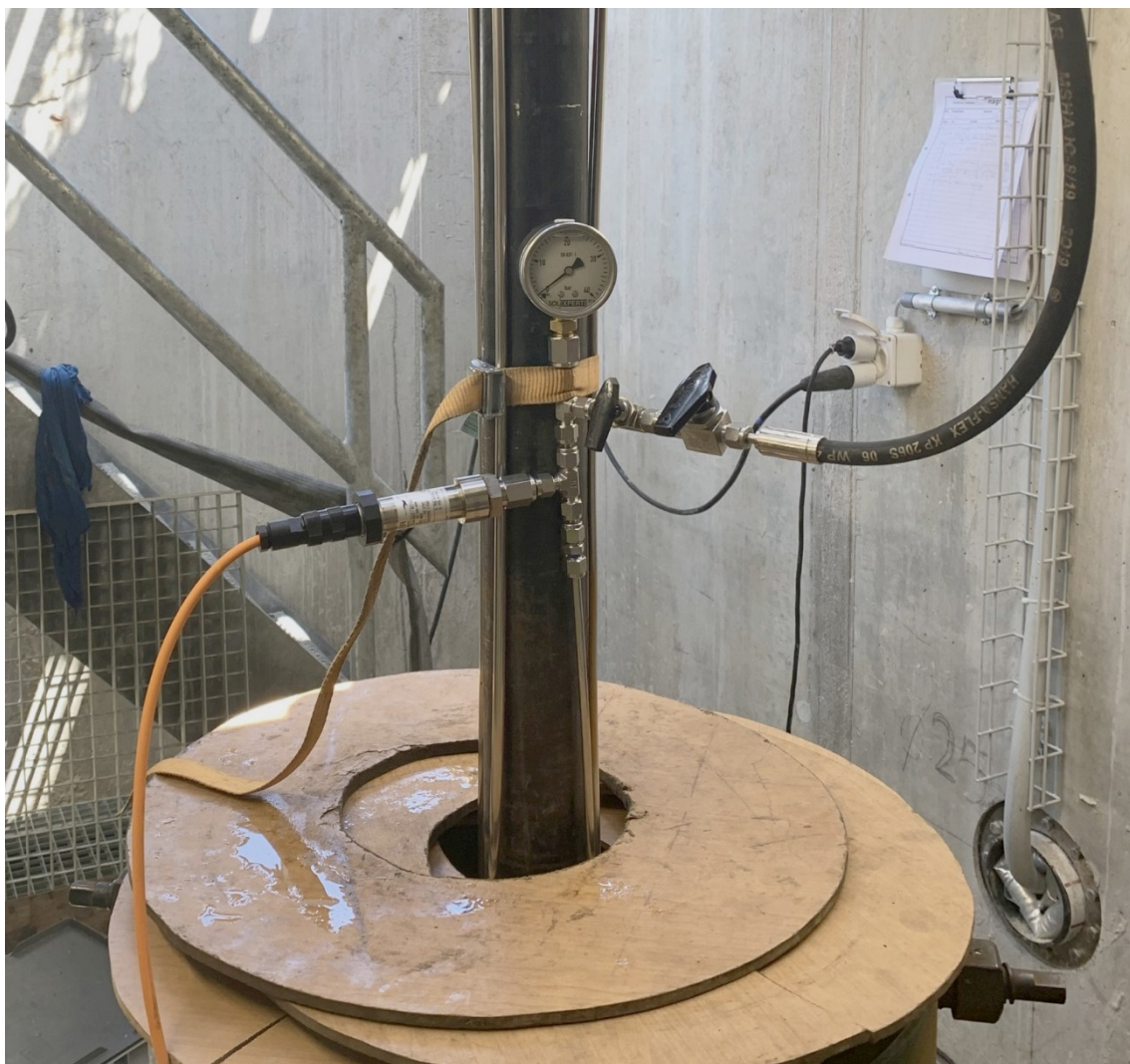
Fig. 3-2: Packer inflation for verification of packer performance inside the borehole The borehole is covered to prevent accidental loss of equipment in the borehole.
