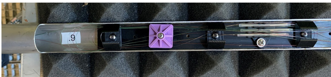
Fig. 2-8: View of the opened splice box with three splices of the FO cable
