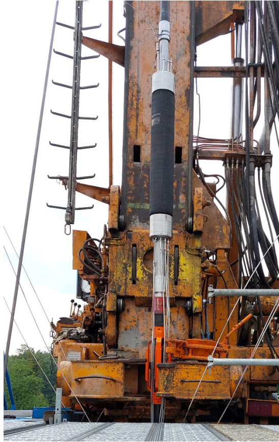
Fig. 2-2: Installation of a packer element on the central tubing with a centralizer below
