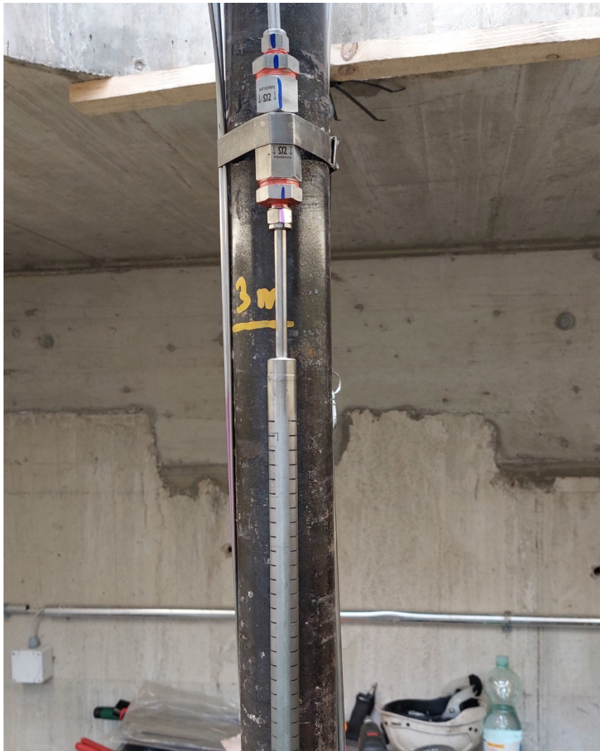
Fig. 2-4: Filter port with burst disc above, installed on the central tubing with metal banding straps
