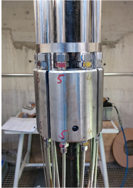
Fig. 2-1: Hanger sub with monitoring and inflation lines below and standpipes above, respectively
