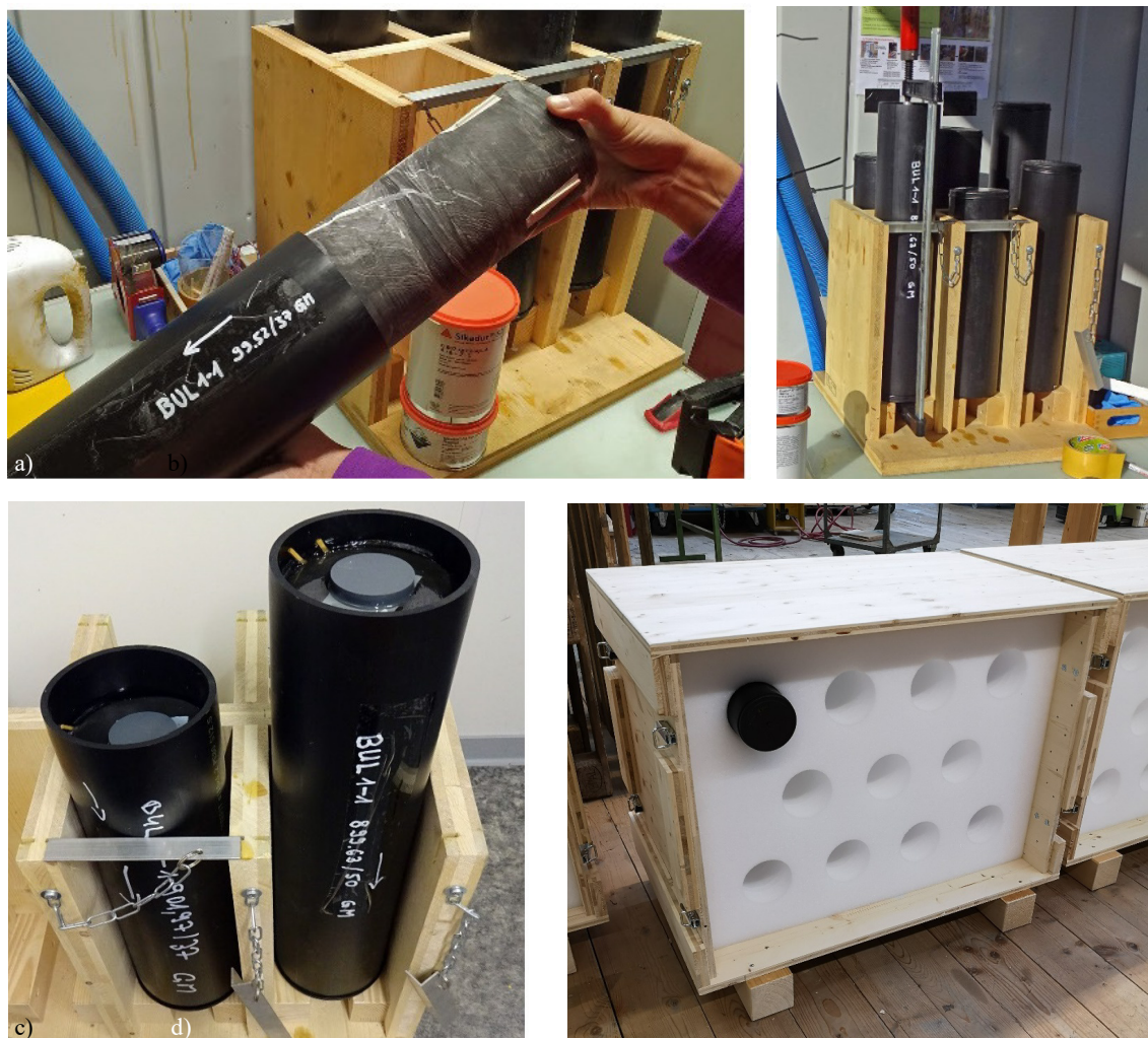
Fig. 3-1: Sampling and storage workflow of GM cores
