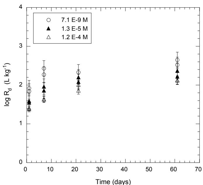
Fig. 6.3: Sorption kinetics of Ni uptake on MX-80 in batch experiments in the porewater composition given in Table 4.2
