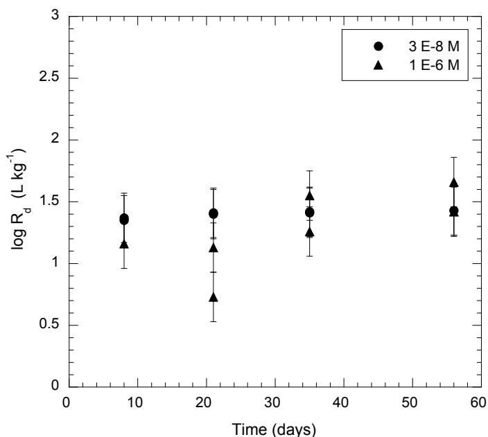
Fig. 6.9: Sorption kinetics of U uptake on MX-80 in batch experiments in the porewater composition given in Table 4.2.
