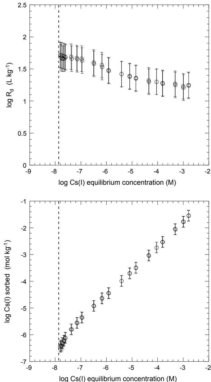
Fig. 6.2: Sorption isotherm of Cs on MX-80 measured in batch experiments in the porewater composition given in Table 4.2. (From Table 4.3 the background concentration of Cs in the EBPW is  $1.2 \times 10^{-8}$  M, indicated by the dashed line.)
