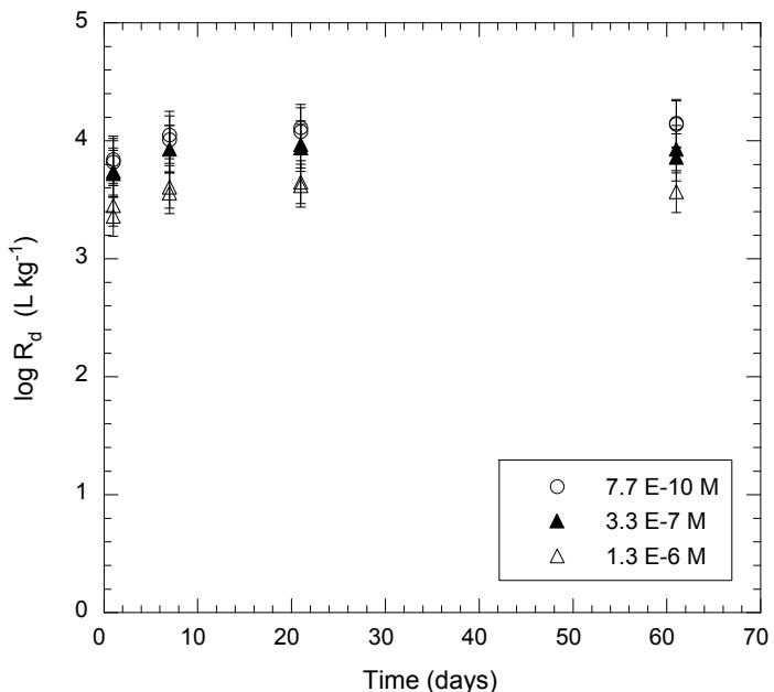
Fig. 6.5: Sorption kinetics of Eu uptake on MX-80 in batch experiments in the porewater composition given in Table 4.2.
