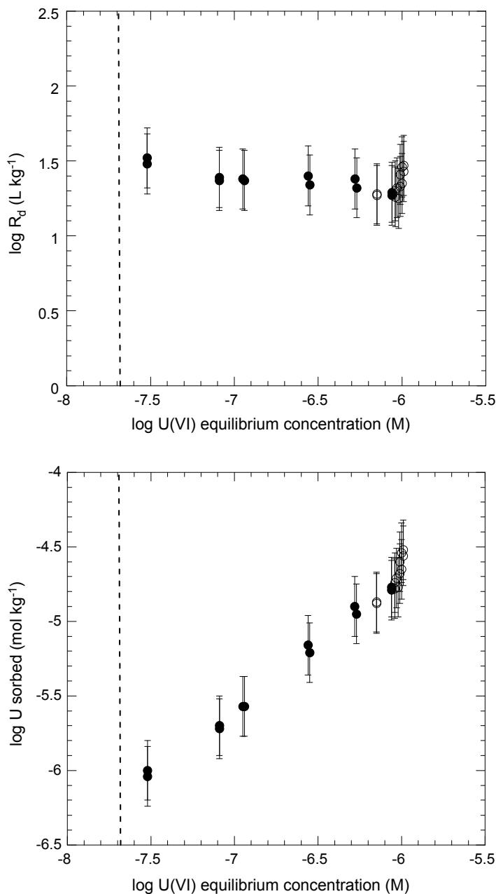
Fig. 6.10: Sorption isotherm of U on MX-80 measured in batch experiments in the porewater composition given in Table 4.2. (From Table 4.3 the background concentration of U in the EBPW is  $2.1 \times 10^{-8}$  M, indicated by the dashed line.)
