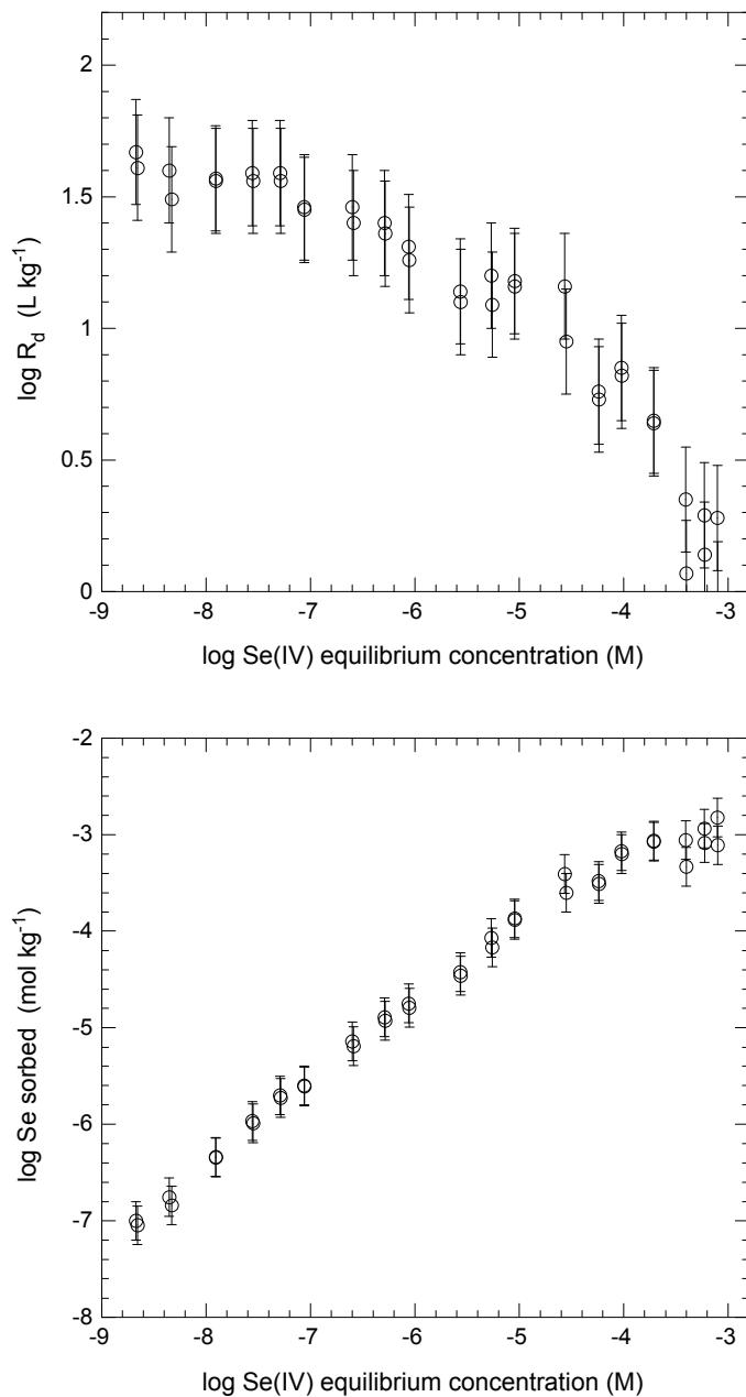
Fig. 6.12: Sorption isotherm of Se on MX-80 measured in batch experiments in the porewater composition given in Table 4.2. (From Table 4.3 the background concentration of Se in the EBPW is  $< 1.3 \times 10^{-7}$  M.)
