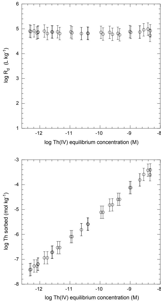
Fig. 6.8: Sorption isotherm of Th on MX-80 measured in batch experiments in the porewater composition given in Table 4.2. (From Table 4.3 the background concentration of Th in the EBPW is  $< 4.3 \times 10^{-10}$  M.)
