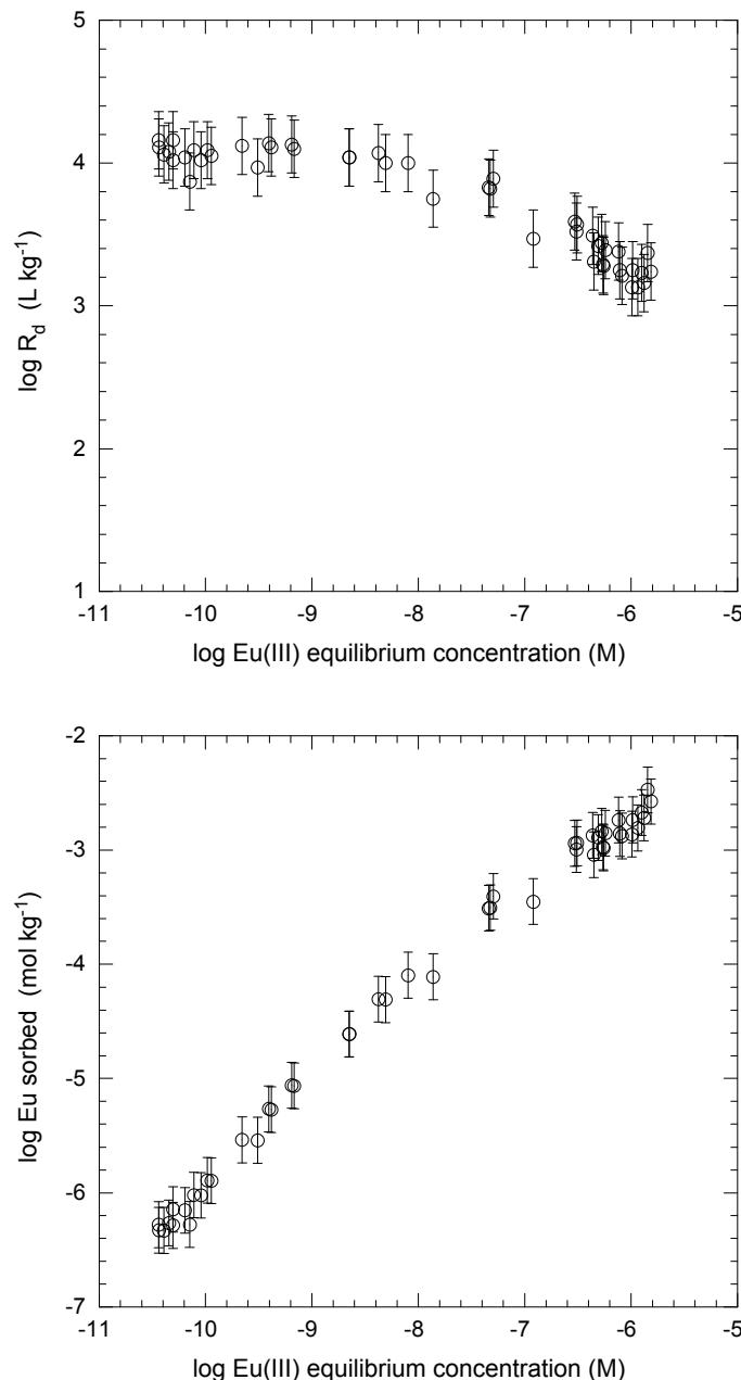
Fig. 6.6: Sorption isotherm of Eu on MX-80 measured in batch experiments in the porewater composition given in Table 4.2. (From Table 4.3 the background concentration of Eu in the EBPW is  $< 3.3 \times 10^{-9}$  M.)
