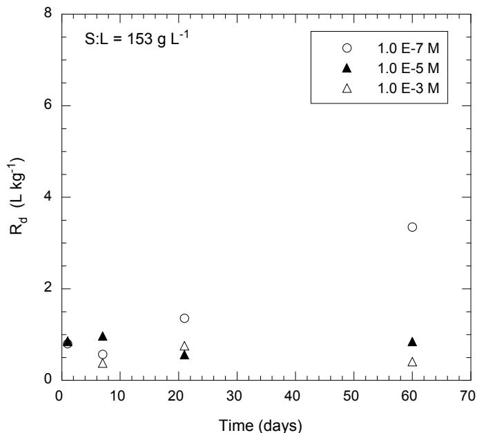
Fig. 6.13: Sorption kinetics of I uptake on MX-80 in batch experiments at 153 g L<sup>-1</sup> in the porewater composition given in Table 4.2.
