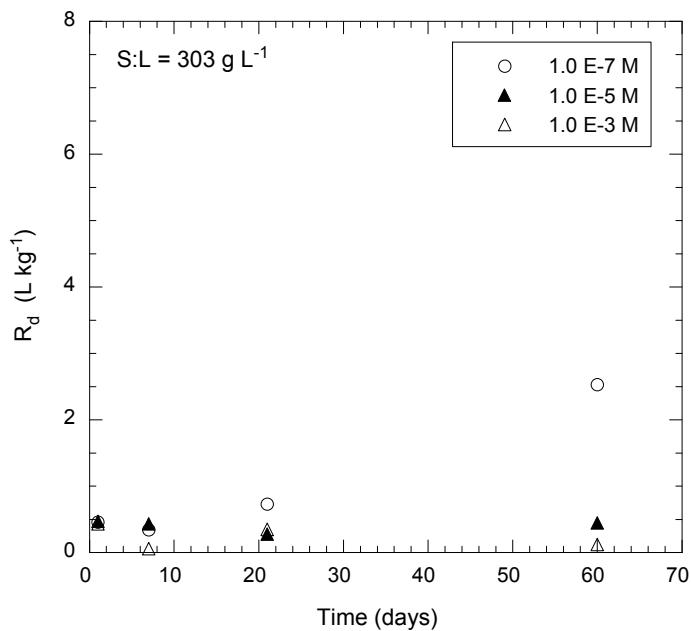
Fig. 6.14: Sorption kinetics of I uptake on MX-80 in batch experiments at 303 g L<sup>-1</sup> in the porewater composition given in Table 4.2.
