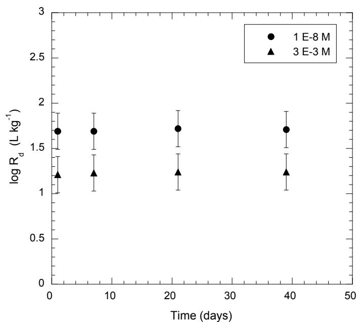
Fig. 6.1: Sorption kinetics of Cs uptake on MX-80 in batch experiments in the porewater composition given in Table 4.2.
