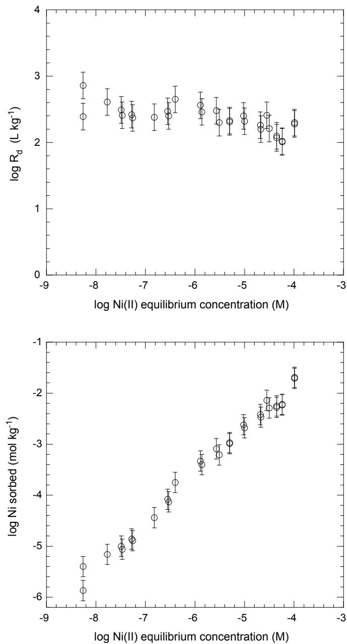
Fig. 6.4: Sorption isotherm of Ni on MX-80 measured in batch experiments in the porewater composition given in Table 4.2. (From Table 4.3 the background concentration of Ni in the EBPW is  $< 1.7 \times 10^{-8}$  M.)
