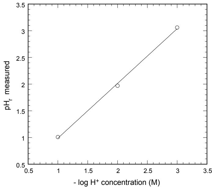
Fig. 5.1: Plot of the measured pH ( $\text{pH}_r$ ) against known proton concentrations in 0.6 M NaCl.
