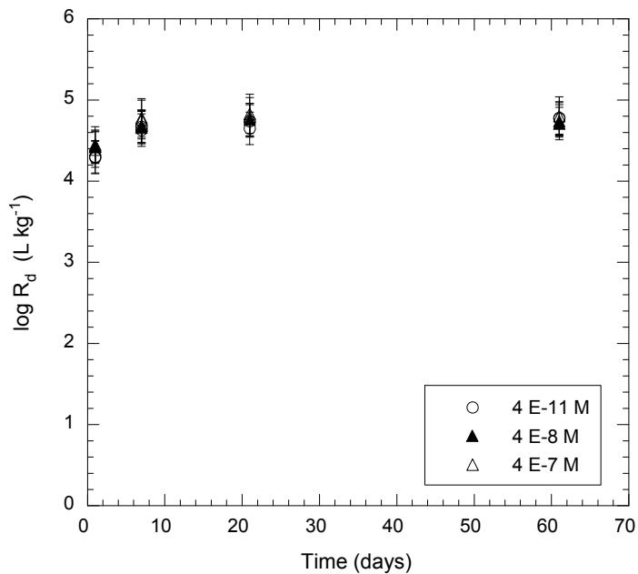
Fig. 6.7: Sorption kinetics of Th uptake on MX-80 in batch experiments in the porewater composition given in Table 4.2.
