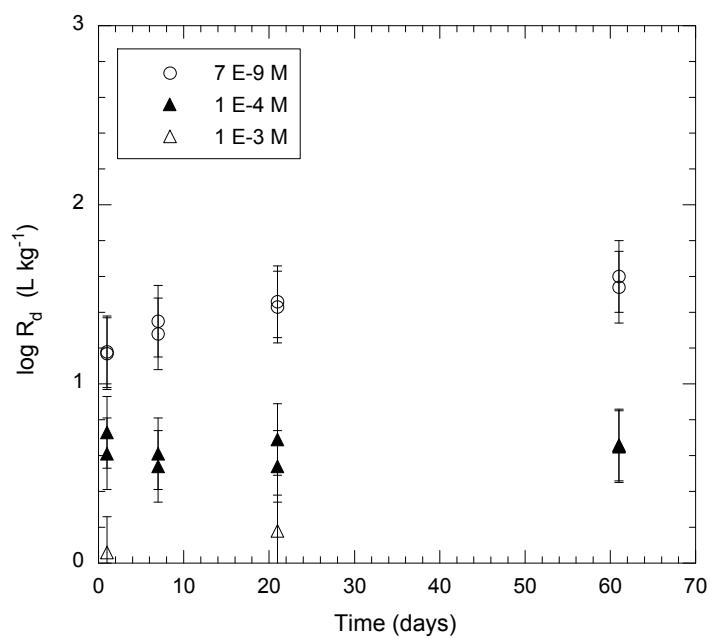
Fig. 6.11: Sorption kinetics of Se uptake on MX-80 in batch experiments.
