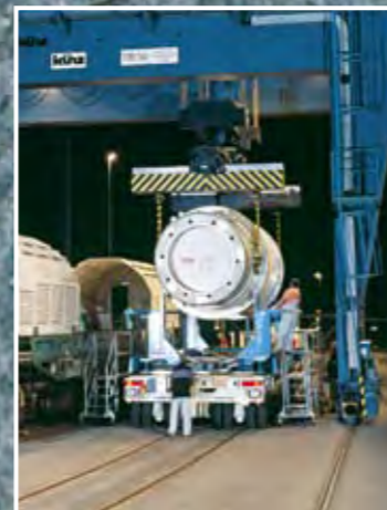
Transport of radioactive waste in Switzerland has been ongoing for many years without any accidents. The photograph shows waste destined for the interim storage facility being loaded from rail to road in Würenlingen.
