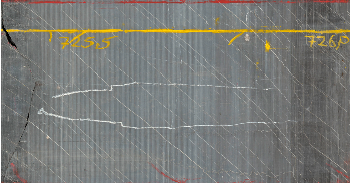
Fig. 3-15: Vein / tension gash
