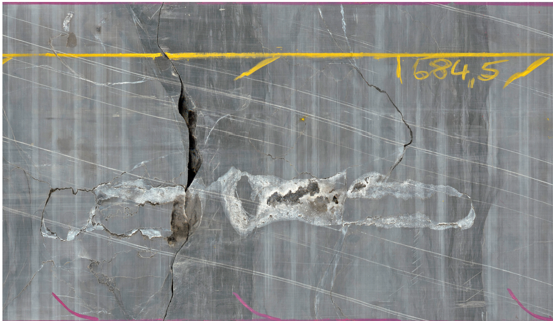
Fig. 3-17: Vein / tension gash
