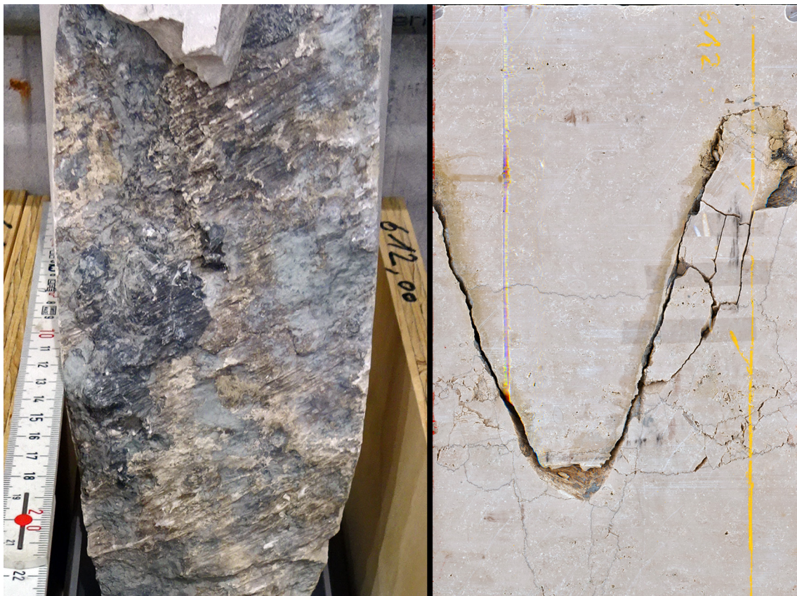
Fig. 3-7: Stylolitic fault plane
