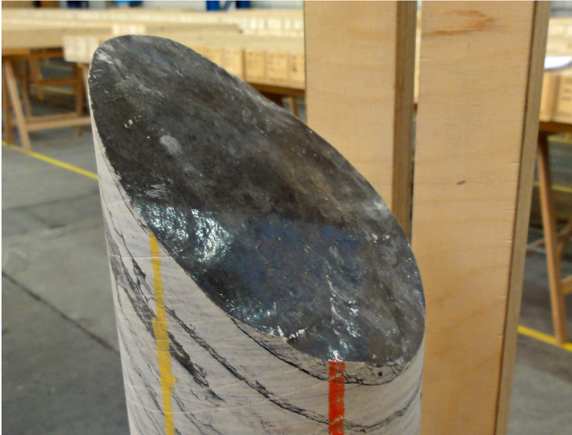
Fig. 3-6: Mirror-like fault plane
