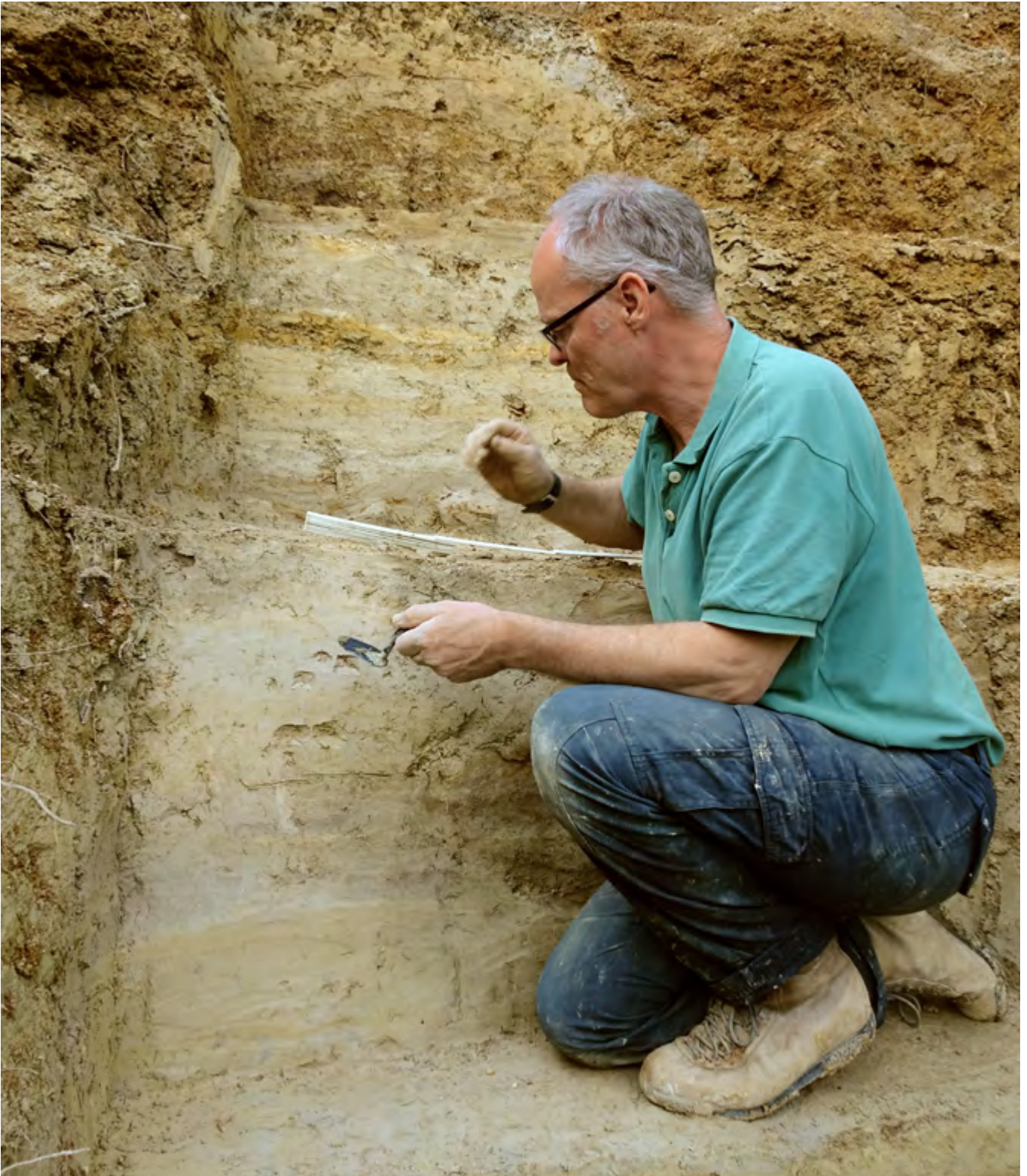
Near Steig above Buch am Irchel (Canton Zürich), Nagra investigated the so-called "Höhere Deckenschotter" ("Upper Cover Gravels") that were deposited there by a former river. The goal was to determine the age of these deposits that lie close to the surface.
