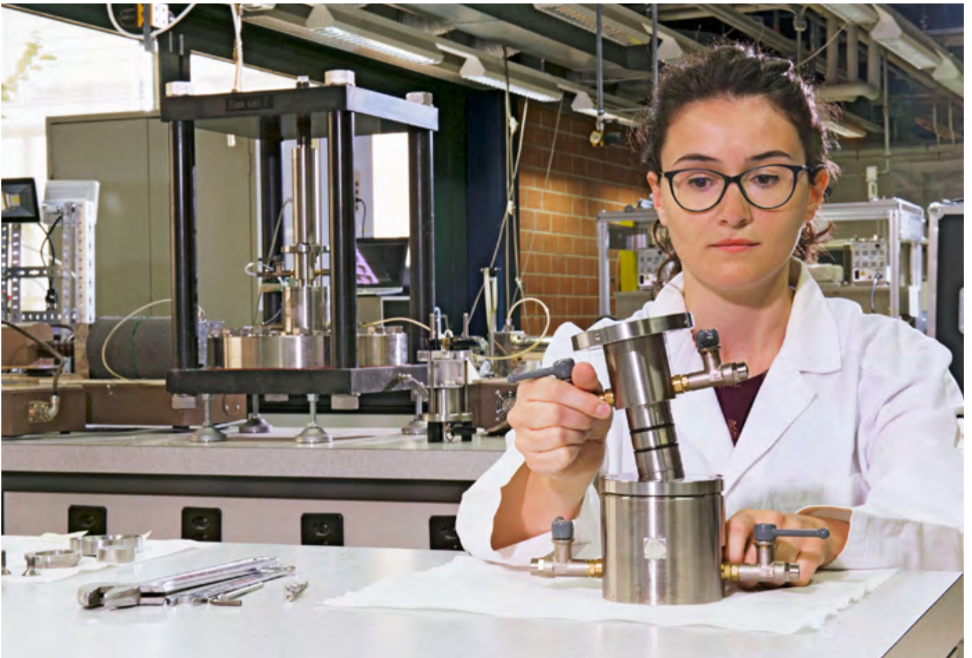
Samples from the deep boreholes are geomechanically investigated at the Swiss Federal Institute of Technology Lausanne (EPFL). With the results of these compression tests, it is possible to estimate the long-term behaviour of the Opalinus Clay when it is subjected to thermal and mechanical stresses.
