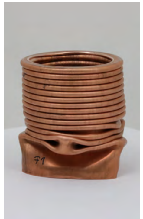
Above: Different bridge plug prototypes are inserted into a borehole where they prevent the longitudinal flow of gases and liquids.
