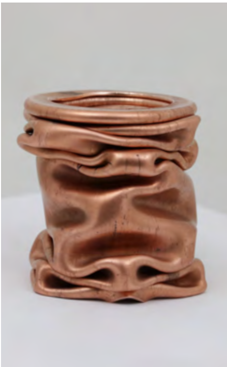
Above: Different bridge plug prototypes are inserted into a borehole where they prevent the longitudinal flow of gases and liquids.
