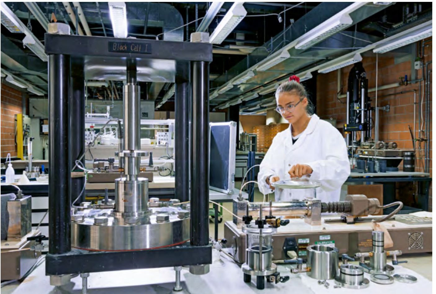
Samples from the deep boreholes are geomechanically investigated at the Swiss Federal Institute of Technology Lausanne (EPFL). With the results of these compression tests, it is possible to estimate the long-term behaviour of the Opalinus Clay when it is subjected to thermal and mechanical stresses.
