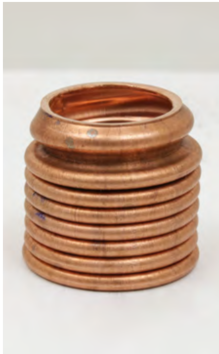
Above: Different bridge plug prototypes are inserted into a borehole where they prevent the longitudinal flow of gases and liquids.
